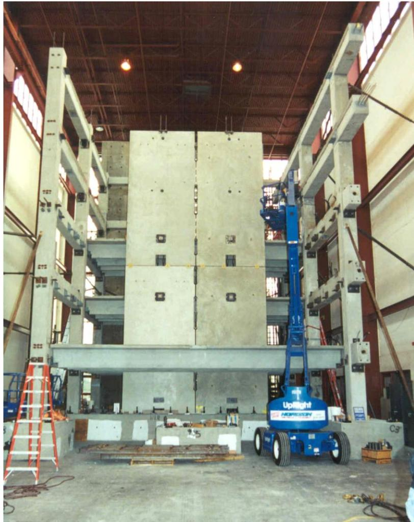
Figure 1.7 The PRESSS building after erecting the wall system (Sritharan et al. 2002)
