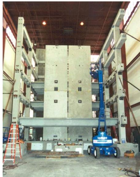
Figure 3.4 The PRESSS test building after erecting the jointed wall system
